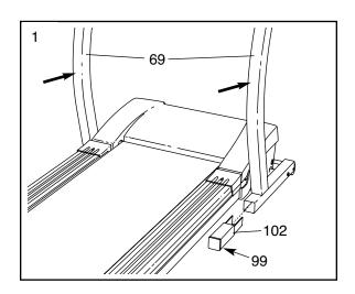
2. With the help of a second person, carefully lower the treadmill frame and then tip the Uprights (69) down as shown. Make sure that the Extension Legs (102) remain in the Uprights.
